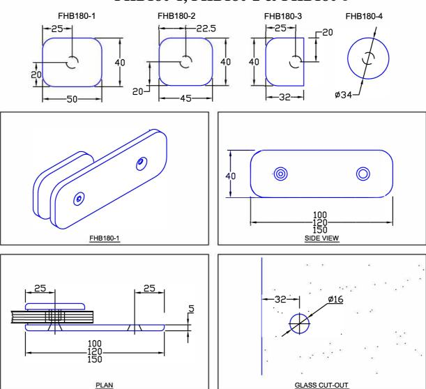
FHB180 Bracket/Clamp Hob to Glass. Manufactured in solid brass designed to secure 180 degree hob to glass shower enclosure panels.
