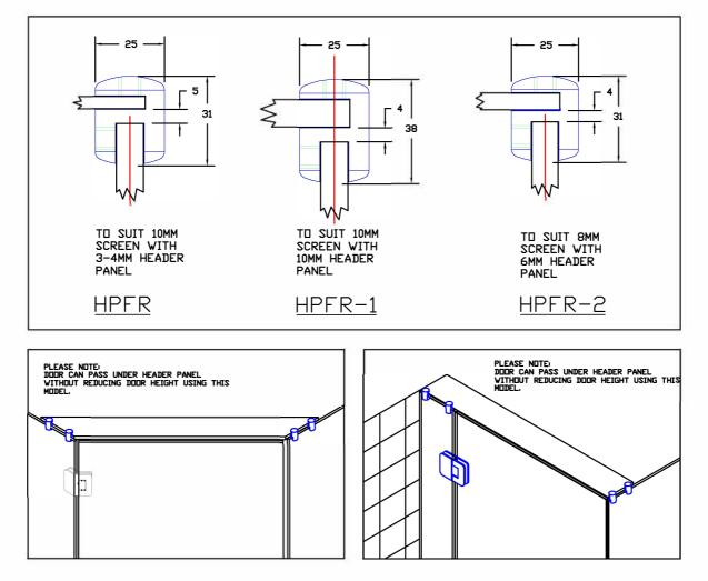
Designed to support frameless glass header panels.
