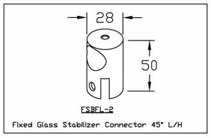
To complete the package for the installation of Frameless Glass Showers the following stabilizers are available. Designed to suit 6mm & 8mm glass but can be adapted to suit various sizes on request.
