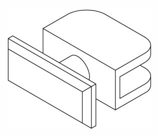
GLASS CUT-OUT IS A SINGLE 16MM DIAMETER HOLE WHERE REQUIRED
