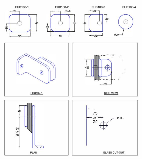
FHB100 Bracket/Clamp Wall to Glass. Manufactured in solid brass, and designed to secure 90 degree wall to glass shower enclosure panels to the wall or floor. FHB100-1,2,3,4 indicates backplate option as shown above.
