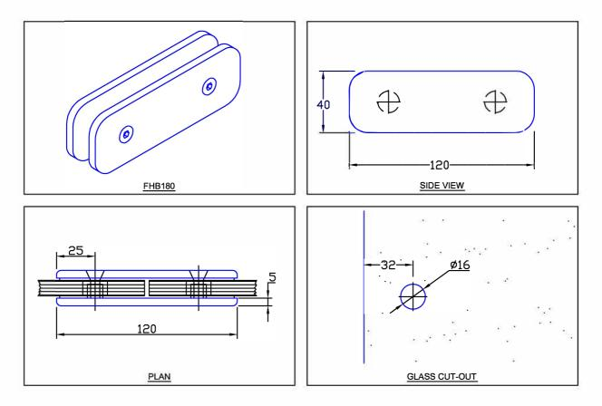
FHB180 Bracket/Clamp Glass to Glass. Manufactured in solid brass designed to secure 180 degree glass to glass shower enclosure panels.
