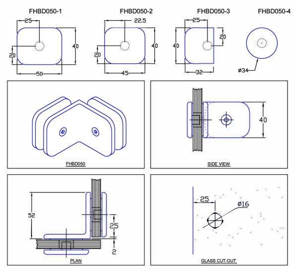
FHBD050 Bracket/Clamp Glass to Glass. Manufactured in solid brass, designed to secure 90 degree glass to glass shower enclosure panels. FHBD050-1,2,3,4 indicates backplate option as shown above.
