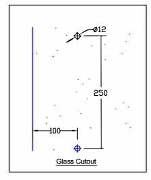
TS25 HANDLE A set consists of one TS25 handle for each side of the glass door.
