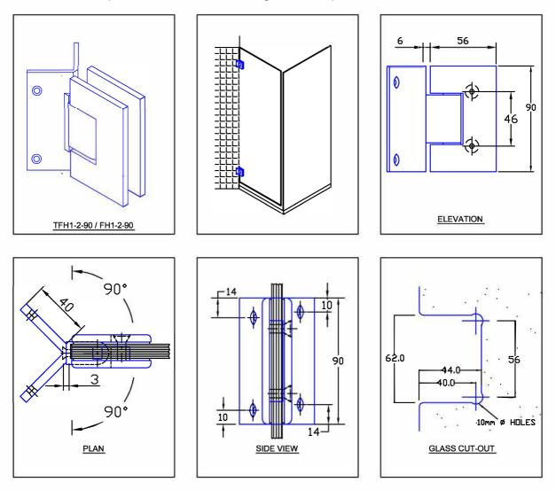
TFH1-2-90 / FH1-2-90 - Wall to Glass corner mounted hinge, on a 90 degree corner
