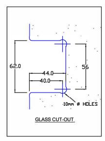
TFH1-2 / FH1-2 Wall to Glass center mounted hinge.
