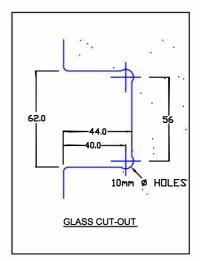
TFH1-2-38 / FH1-2-38 and TFH1-2-50 / FH1-2-50 Wall to Glass side mounted hinge, with two back plate options. 38mm and 50mm.
