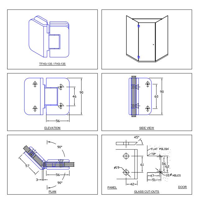
TFH3-135 / FH3-135 Glass to Glass hinge to mount a door to a fixed glass side panel that runs at a 135 degree angle. The hinge is secured to the panel with two holes in the glass instead of a cut-out. This results in a simpler and cheaper glass preparation. Additional advantages are better holding capabilities, and a cost effective hinge.
