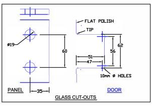
TFH3-180 / FH3-180 Glass to glass hinge to mount a door to a fixed glass side panel that runs on a 180 degree plane. The hinge is secured to the panel with two holes in the glass instead of a cut-out. This results in a simpler and cheaper glass preparation. Additional advantages are better holding capabilities, and a cost effective hinge.
