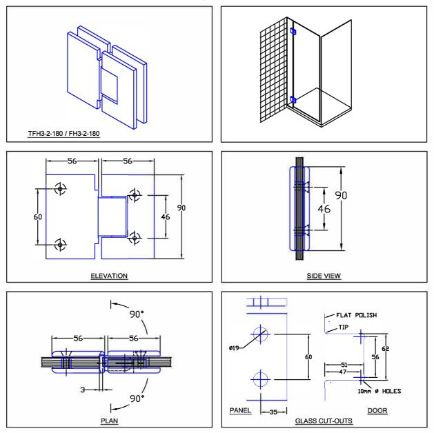
TFH3-2-180 / FH3-2-180 Glass to glass hinge to mount a door to a fixed glass side panel that runs on a 180 degree plane. The hinge is secured to the panel with two holes in the glass instead of a cut-out. This results in a simpler and cheaper glass preparation. Additional advantages are better holding capabilities, and a cost effective hinge.
