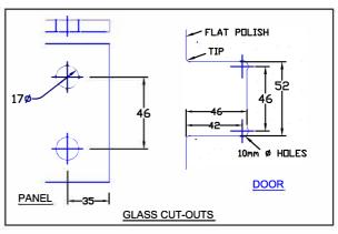
FH3-6-180 Glass to glass hinge to mount a door to a fixed glass side panel that runs on a 180 degree plane. The hinge is secured to the panel with two holes in the glass instead of a cut-out. This results in a simpler and cheaper glass preparation. Additional advantages are better holding capabilities, and a cost effective hinge.
