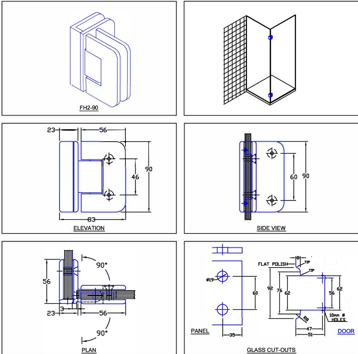
FH2-90 Glass to glass hinge to mount a door to a fixed glass side panel that runs on a 90 degree angle. The hinge is secured to the panel with two holes in the glass instead of a cut-out. This results in simpler and cheaper glass preparation . Additional advantages are better holding capabilities, and a cost effective hinge.
