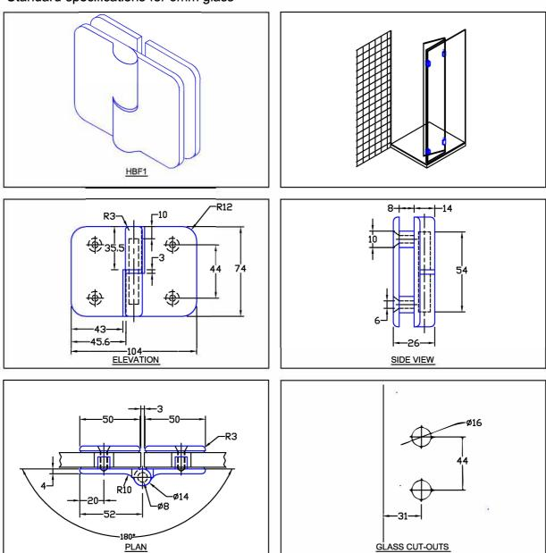
HBF1 Glass to Glass hinge to mount a door to a 6mm glass side panel. This Bi-Fold hinge has the advantage of allowing the glass to fold back on itself through a 180° angle. The hinge is secured to the panel with two holes in the glass instead of a cut-out. This results in a simpler and cheaper glass preparation. Additional advantages are better holding capabilities, and a cost effective hinge.
