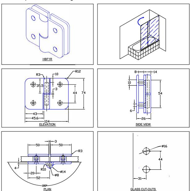
HBF1R Glass to Glass hinge to mount a door to a 6mm glass side panel. This Bi-Fold hinge has the advantage of allowing the glass to fold back on itself through a 180° angle. The hinge is secured to the panel with two holes in the glass instead of a cut-out. This results in a simpler and cheaper glass preparation. Additional advantages are better holding capabilities, and a cost effective hinge.
