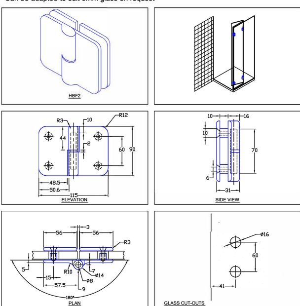
HBF2 Glass to Glass hinge to mount a door to a 8mm or 10mm glass side panel. This Bi-Fold hinge has the advantage of allowing the glass to fold back on itself through a 180° angle.
