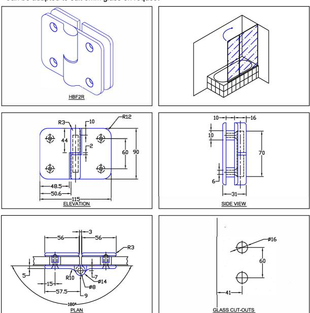
HBF2R Glass to Glass hinge to mount a door to a 8mm or 10mm glass side panel. This Bi-Fold hinge has the advantage of allowing the glass to fold back on itself through a 180° angle.
