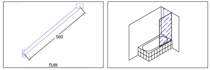
BBS. Stabilizer/Bracket Wall to Glass. Manufactured in solid brass and designed to secure fixed bath shower enclosure glass panels. The bracket is secured to the glass by a nylon tipped grub screw. Designed to suit 6mm, 8mm & 10mm glass, but can be adapted to suit various sizes on request.
