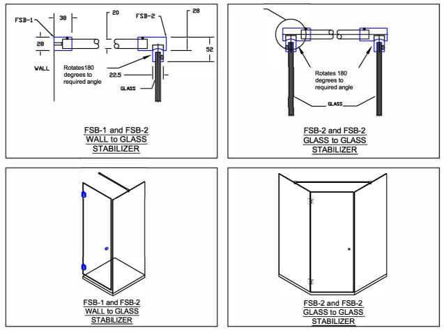
Top fixed Stabilizer Bars to reduce glass panel movement. Fittings available for wall to glass and glass to glass. Angle is 180 degree adjustable. Designed to suit 8mm & 10mm Glass.
