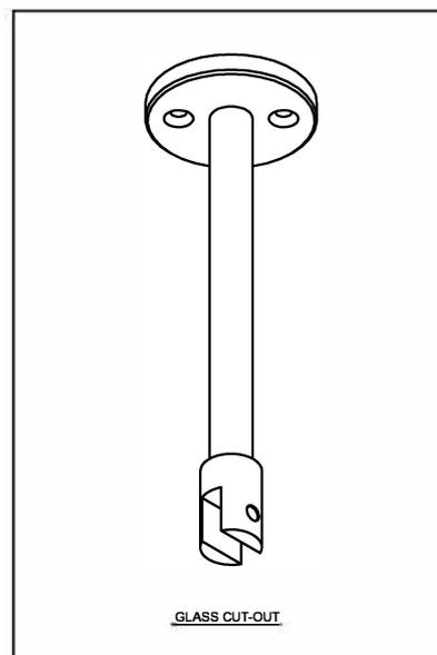
Roof to glass stabilizer bars can also be used as floor to glass pedestal supports.
